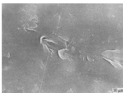
Figure 4. SEM of a cryo-fractured (10/90) LDPE/PS blend, compatibilized by 10 wt.% EBS-3.
